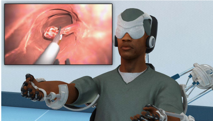
Figure 1.7: The TeleFLEX project focusses on an intuitive tele-manipulation system for surgical interventions with flexible instruments.
