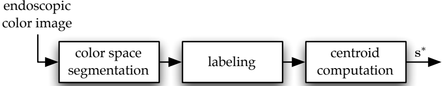
Figure 4.5: Endoscopic image processing: From the endoscopic image, the marker regions are extracted and their centroids are computed.
